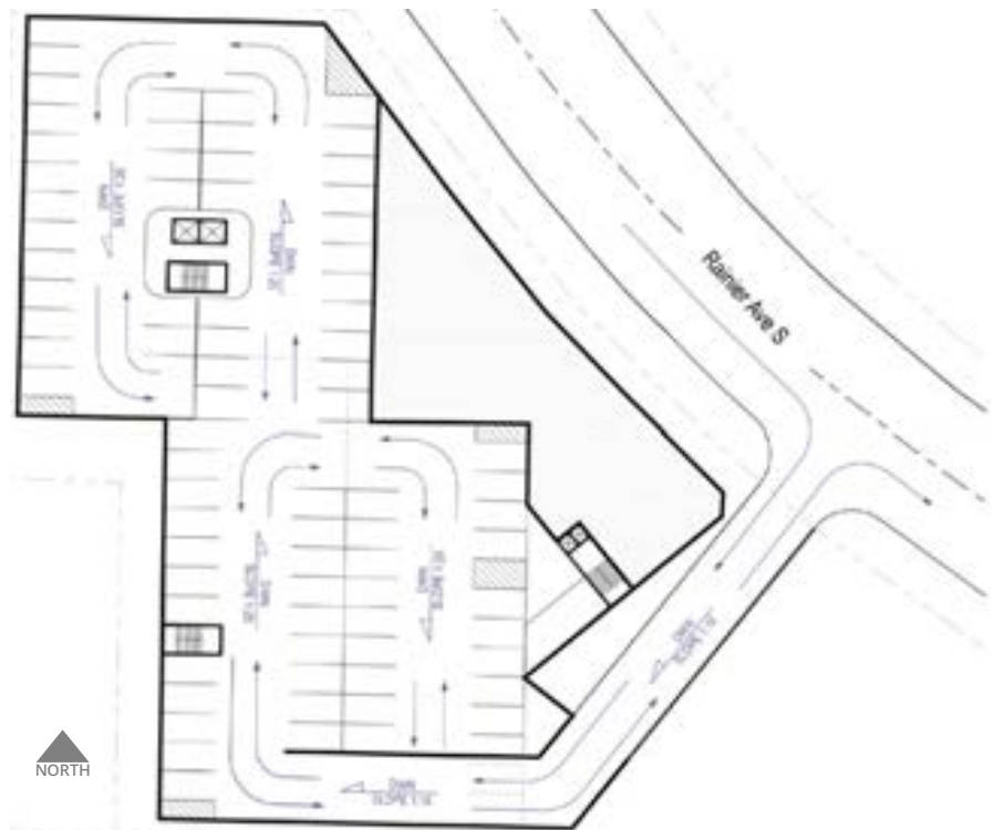
Underground parking garage provides 100 parking stalls.
