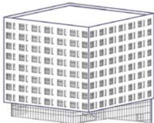
Phase 3: The proposed NE corner building has a split-level ground floor with shared spaces for church and community use plus 8 floors of apartments.
